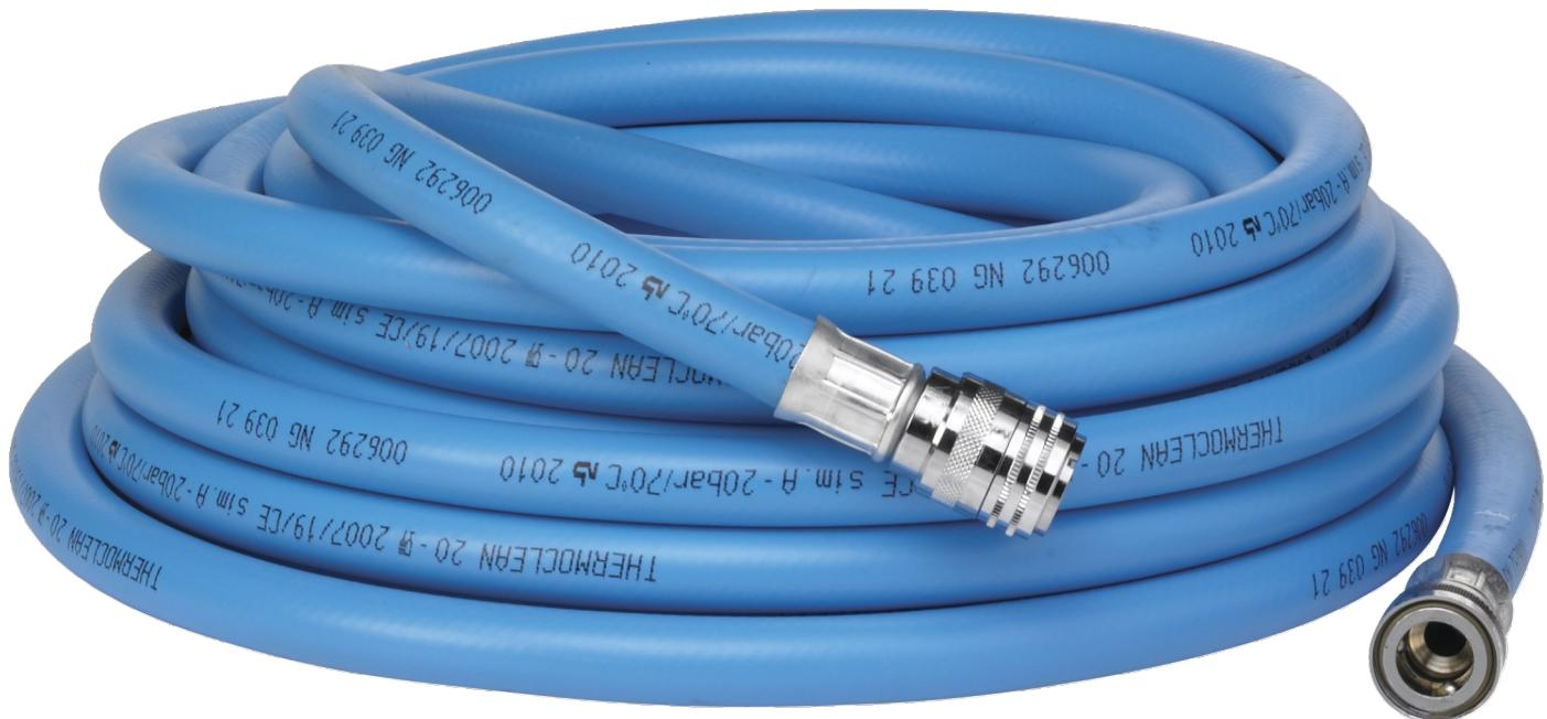
This Hot Water Hose is ideal for cleaning with water up to 70° C. It is equipped with a 1/2" Q-coupling in both hose ends. Water tap nipple, 0700 provided for 1/2", 3/4" and M22x1 screw thread types. Can be used with the following Vikan Q-couplings 0700, 0705 and 0712 as well as other Vikan products equipped with a 1/2" Q-nipple.
